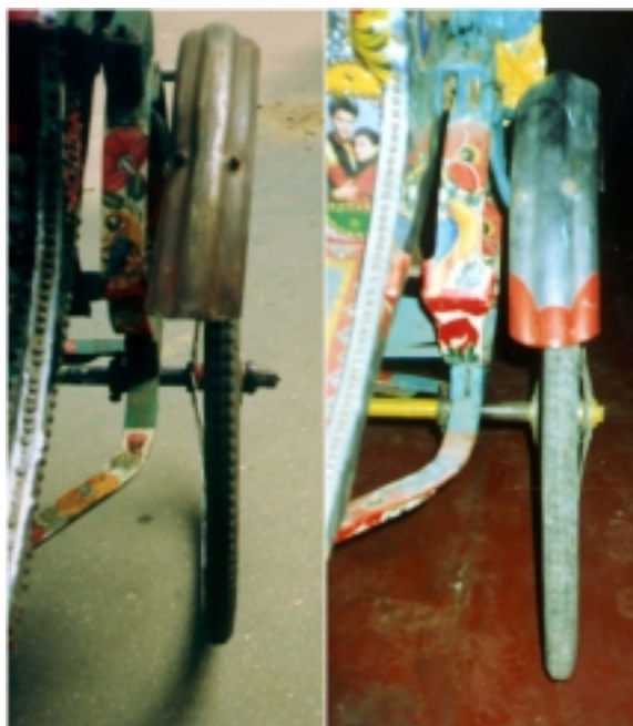
Fig.5 Rear axle with wheel. Present design at the left and modified design at the right, reduced overhanging of shaft beyond the wheels.
